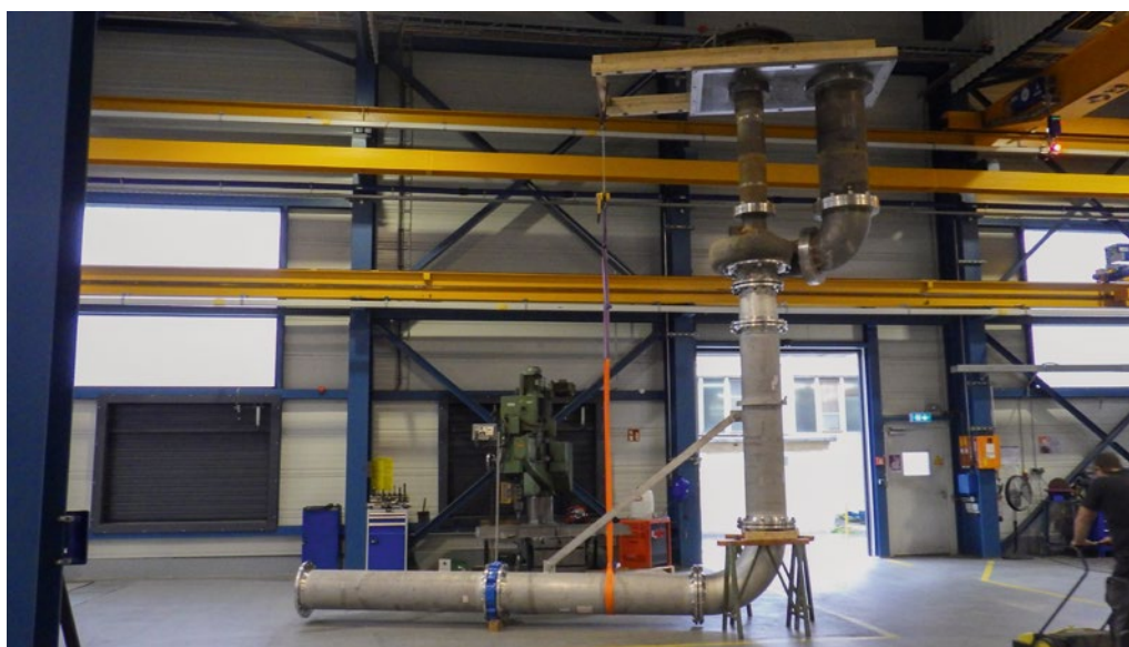
In 2013, the company installed the NPSH measurement setup of the prototype on the test bench.
