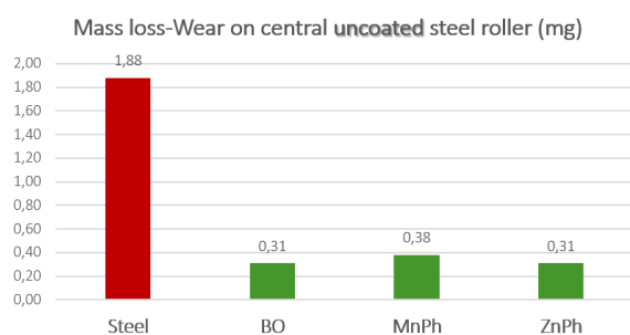
Figure 7: MPR wear test results – mass loss of the steel roller in contact with different uncoated (steel) and coated rings
