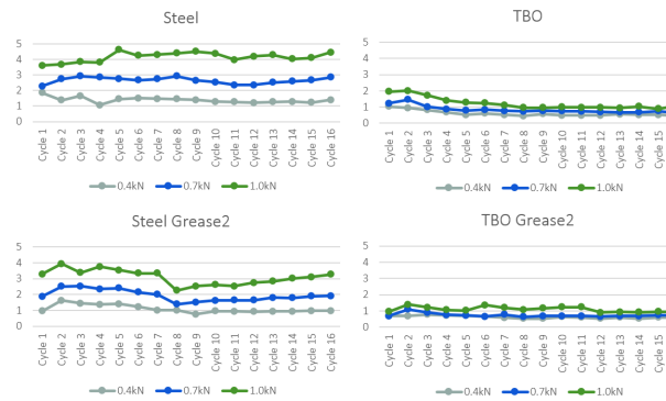
Figure 6: Time evolution of relative frictional torque for different axial loads at 1800 rpm
