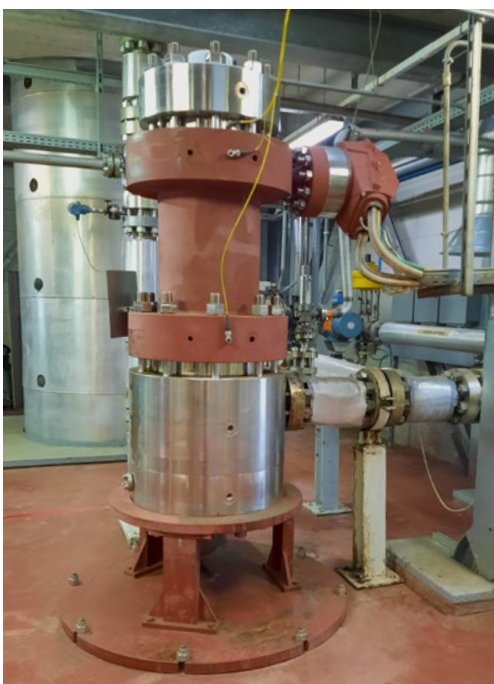
Vertical canned motor pump in high pressure design.
